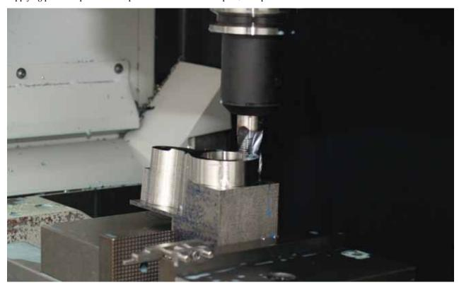
Complex lever is machined from titanium in three setups on a Mazak Variaxis 500 five-axis VMC allowing a single vise setup for this sculptured lever, versus nine setups using traditional processes.
