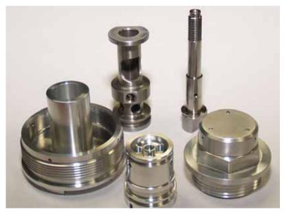
Many families of round parts requiring secondary milling, drilling, and tapping operations are completely processed in a Mazak Integrex Multitasking center.
