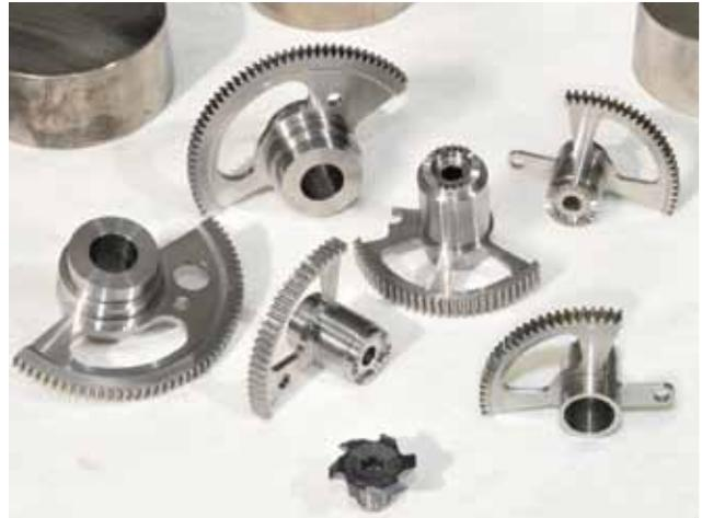
***Sector gear, machined from solid 17-4PH bar stock, looks like half a gear with a lever arm attached. Measuring about 3½" (89-mm) diameter with 46 teeth over a 180° arc, the gears produced by ASPI go into helicopter flight controls.***
