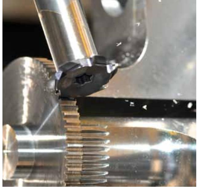
***Modified standard Chip-Surfer slotting tool forms teeth in just two passes, shaving 20 minutes off tooth-forming cycle time for this sector gear at ASPI. Eliminated is the tooling baggage usually associated with gear-tooth machining. No swapping out HSS gear gashers or dealing with regrinds. Operator simply changes tips in seconds and starts up again.***
